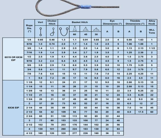
Rated Capacities in Basket Hitch based on D/d Ratio of 25.
